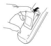
2. Place the two accessory R6P (SUM-3)/AA (15F) batteries in the remote control according to the polarity markings ("+" and "-") inside the compartment and on the batteries.
